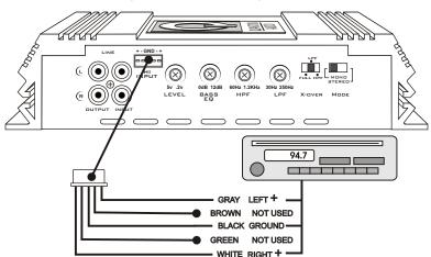
TWO CHANNEL CONNECTIONS: COMMON GROUND RADIO
